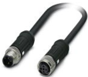
Sensor/Actuator cable, 3-position, PE-X halogen-free, black, shielded, Plug straight M12 SPEEDCON, A-coded, on Socket straight M12 SPEEDCON, A-coded, Cable length: 5 m, For railway applications
